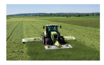
Attachments such as mowers often protrude far beyond the front and rear of the tractor and block the driver's view.
