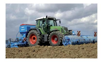
Large seed drills can obstruct the tractor driver's view of the area behind the tractor or the tractor/trailer pair.
