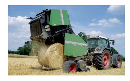
The bale ejection cannot be seen from the driver's seat. The MC7000 series cameras allow the driver to detect faulty operations in a timely manner.
