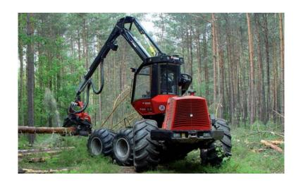
Due to the enormous machine size, the drivers of wood harvesters frequently lack a sufficient all-round view for safe manoeuvring.
