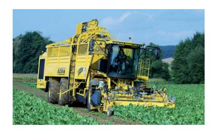
A camera system on beet harvesters consists of up to four cameras. They capture the area behind the machines and monitor the star strainers and conveyor belts inside.
