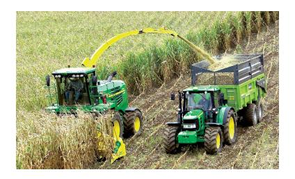
The drivers of additional tractors on the edge of the field can receive the camera image of the discharge curve and thus ensure an efficient transport chain.
