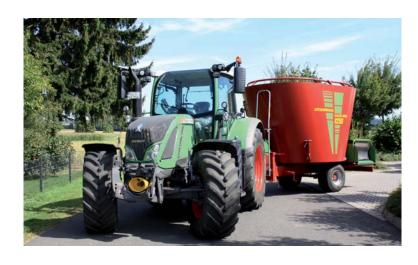
The large size and shape of feed mixers generally block the driver's rear view. The mounted mirrors do not offer an adequate field of vision for this.
